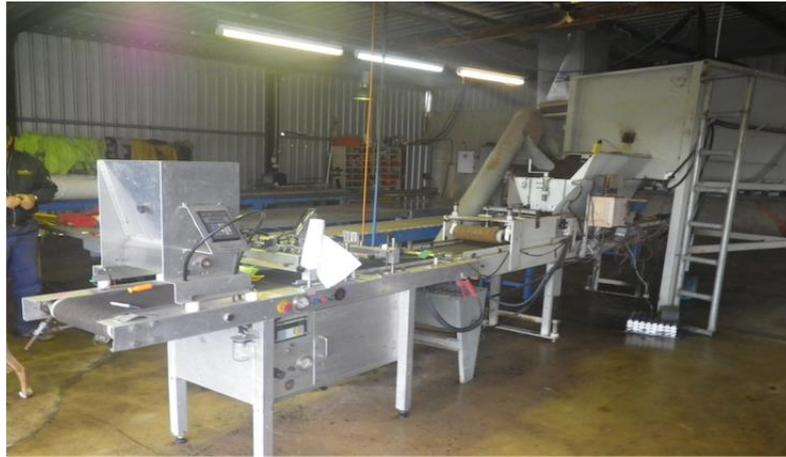
Figure 5: Seed sowing machine in cell tray (Western Australia)
